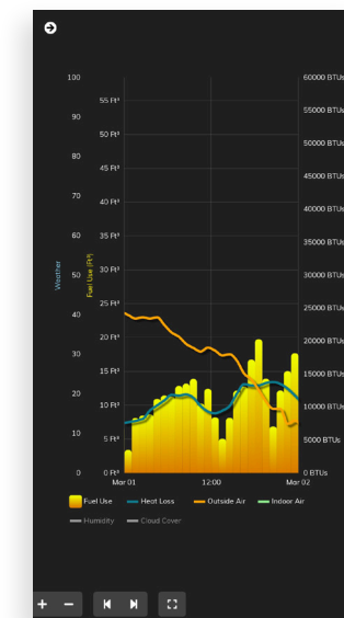
Hourly Fuel Use and Heat Loss: 90 days of accurate hourly building heatloss and energy use compared to inside and outside temperatures
